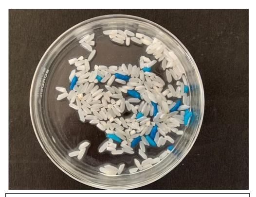
Fortified Rice turning blue on reaction with ferricyanide indicating presence of iron in Fortified Rice Kernel
