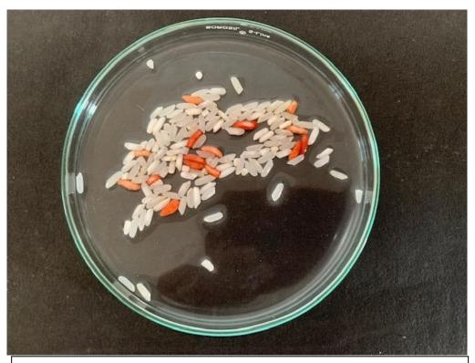
Fortified Rice turning red on reaction with KSCN indicating presence of iron in  $\,$  Fortified Rice Kernel  $\,$
